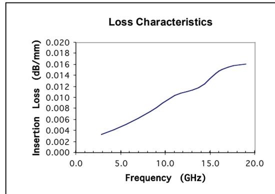
\* Data obtained from measurements on ring resonators. Metallization is co-fired 903-A silver.
